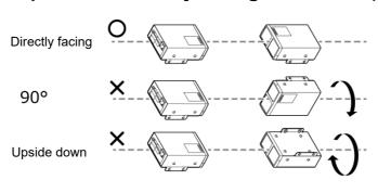
If the installation angle is not aligned, the transmission distance may become reduced and cause transmission failures
