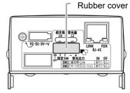
Remove the rubber cover from the LAN connector side and set the switches.
